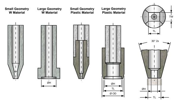
The rather simple geometry of a standard RT tool is frequently adapted to meet more specific requirements. Ultra-thin die or MEMS containing delicate structures, like membranes or air gaps, must be handled with more sophisticated tools. Multi-holes or porous tip material, together with diverse vacuum distribution designs, belong to this tool category.
