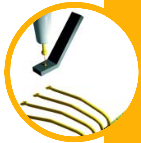
FAB formation during wire bonding process
